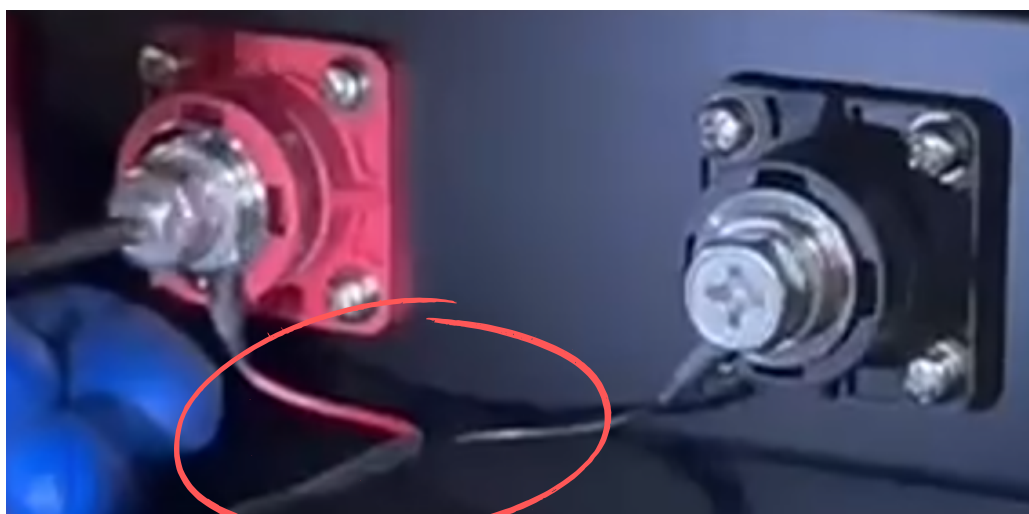
The 2P Cables are pre-connected to the Power Input Socket at the factory
